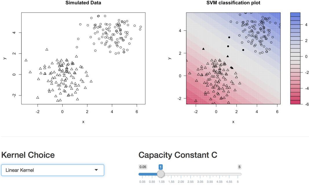
Figure 1: SVM classification (with linear kernel and C = 1 ) on simulated data. 100 points are simulated from a Normal( [0, 0]^T, I ) distribution (where I denotes the 2 \times 2 identity matrix) and labeled as triangles. Another 100 points are simulated from a Normal( [4, 4]^T, I ) and labeled as circles. The left panel shows a scatterplot of the simulated data. The right panel shows the SVM classification. The filled triangles and the filled circles represent the support vectors.
